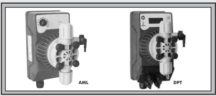
Dayliff Seko Kompact chemical dosing pumps are high specification products for the accurate dosage of a wide range of chemicals in general water treatment and industrial process applications. They are of positive displacement diaphragm type with microprocessor based magnetic solenoid motors.
